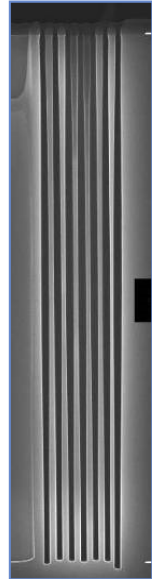
High Aspect Ratio 1.7 x 41 μm 24:1 AR
